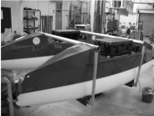
Figure 2a: Springer's USV showing clearly the pelicanses in the bay area between the cross beams
